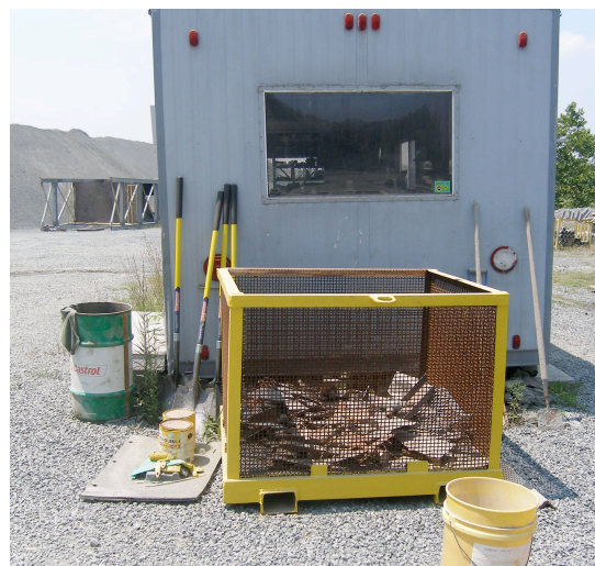
Figure 6. Basket for storing metal scrap that can be moved with a forklift.
