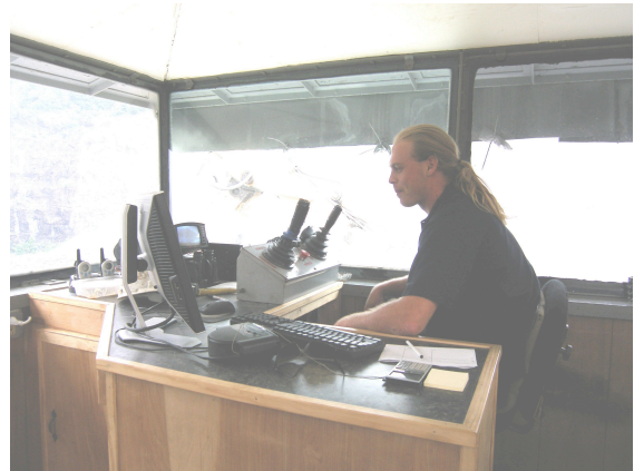
Figure 5. Sitting workstation installed for crusher operator.
