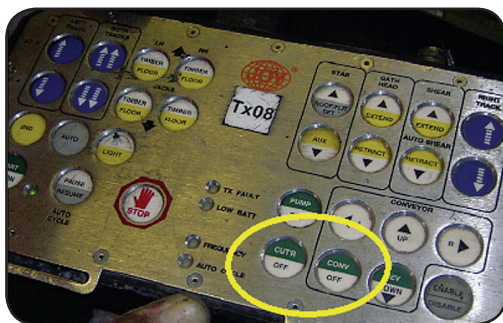
The proximity of conveyor and cutter switches creates a risk of incorrect operation
