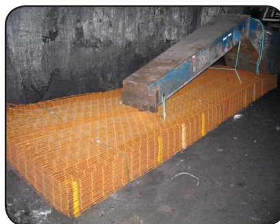
Jib used to load mesh via LHD
