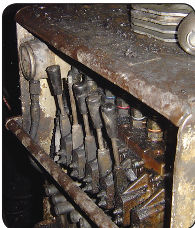
Shape coding through a missing knob
