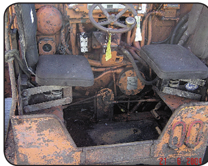
Poor shuttle car seat suspension
