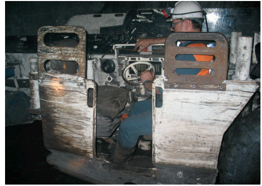
Photo 6: Taller worker operating a shuttle car still with obstructed viewing angles and limited knee room
