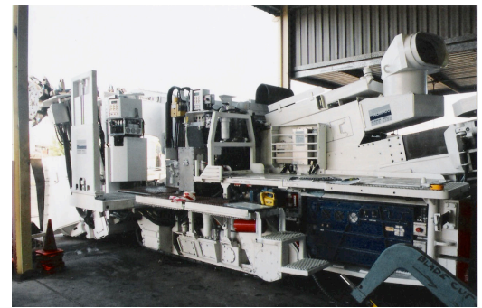
Photo 2: Refurbished Miner – raised and extended floor to assist roof bolting
