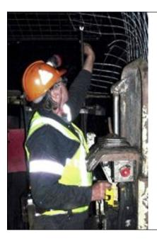
"The bolter rotation and bolter raise control handles are located beside each other but are differing shaped handles. *The handle shape was not consistently applied to all control stations on the machine*...
