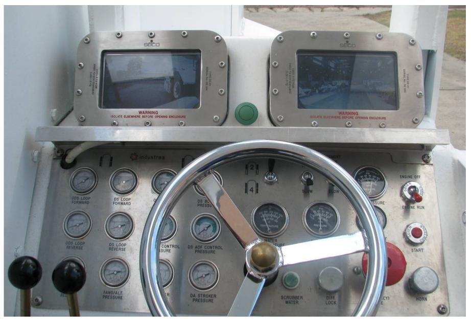
Control Panel with Camera assisted vision. Rear facing camera in mirror configuration
