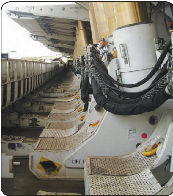
Reduced tripping hazards on front walkway
