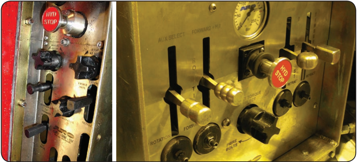
Shape coding of bolting controls
