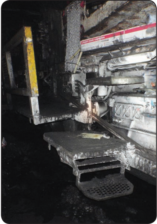
Step access and handrails
