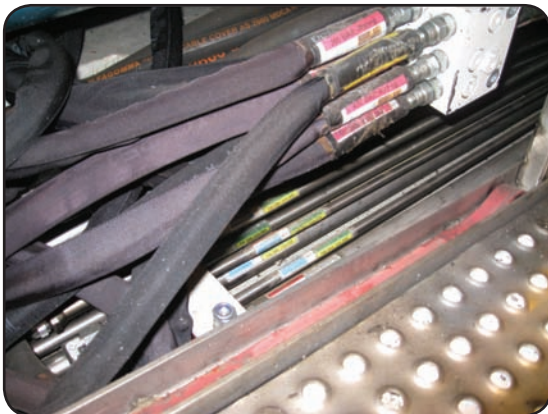
Replacing hydraulic hoses with stainless steel piping where possible
