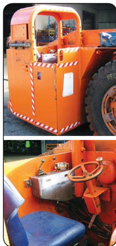
East-west cab fitted to shuttle car (Beltana)
