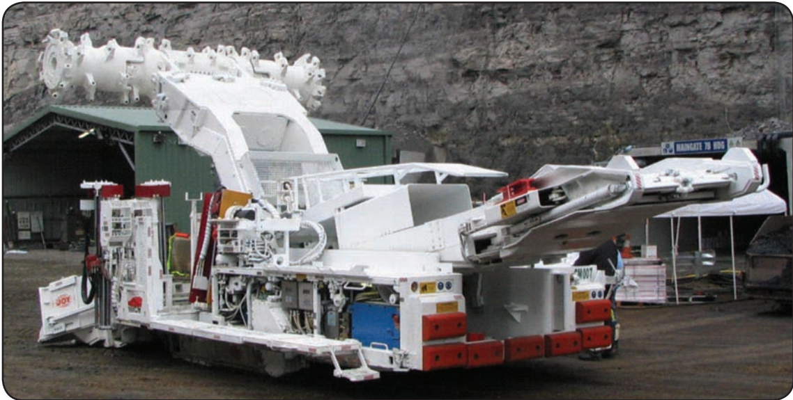
Single level platform and rear step
