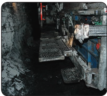
Hinged platform and access step
