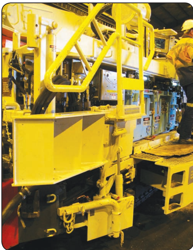
MB650 steps folded for breakaway
