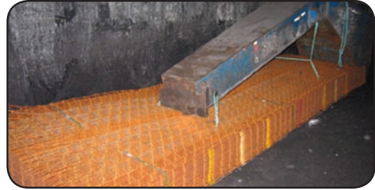
Jib used to load mesh via LHD (Oakly North)
