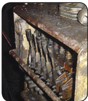
Shape coding through a missing knob
