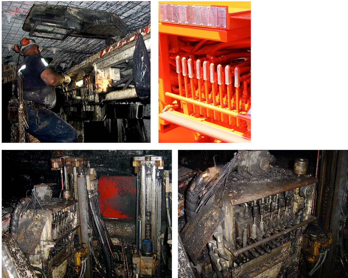
Fig. 1. Examples of bolting rig controls. The controls illustrated in the top of the figure are on a stand-alone bolting machine; those on the bottom are for bolting rigs located on a continuous mining machine (an integrated bolter-miner).
