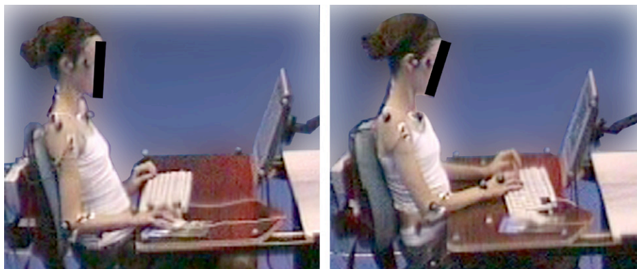
Fig. 1. Workstation setup showing no support and support conditions.
