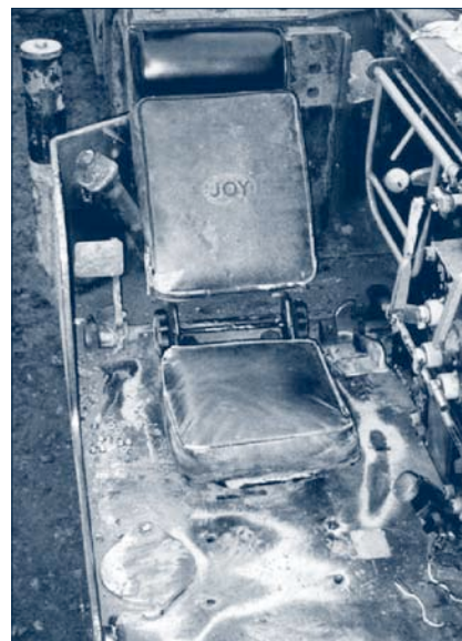
Fig 2. NIOSH Design Mid-Seam Shuttle Car Seat
