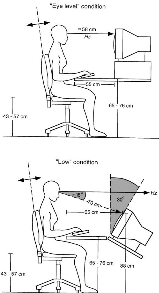
Fig. 1. Workstation layout in "Eye level" and "Low" monitor conditions.
